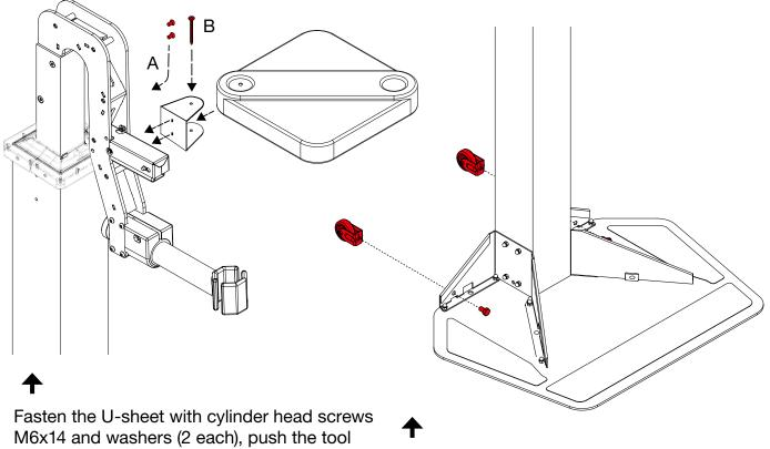
M6x14 and washers (2 each), push the tool tray into the U-sheet and screw it with cylinder head screw M6x90.
