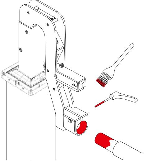
To work particularly efficiently, set the holding clamp almost vertically and lift the bike up by its saddle and fasten the clamp.
