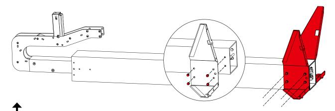
Fix the right/left support bracket and the U-sheet tool tray with cheese-head screws and washers (8 each).
