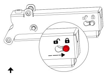
Now take the operating unit and move the locking bolt into the locked position ("Lock closed" symbol).
