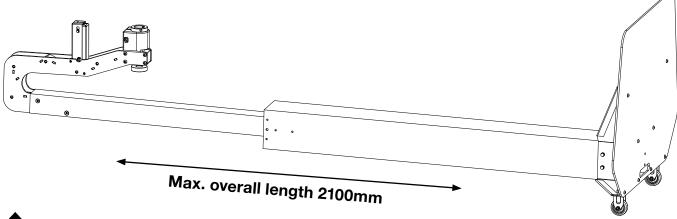
Beware! The piston rod can extend a maximum of 800 mm (max. overall length 2100 mm). Select the location for the assembly so that the repair stand can be laid out completely.
