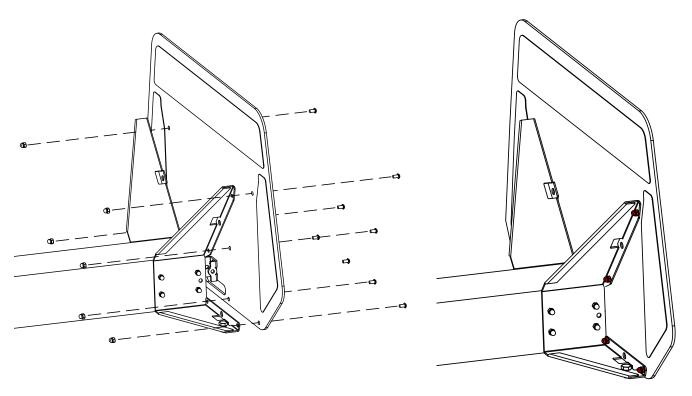
Bring the base plate (1) into its final position to the supporting brackets (1) and then screw them to each other using the oval-headed screws and cap nuts. Then screw the supporting brackets to the external guiding tube.
